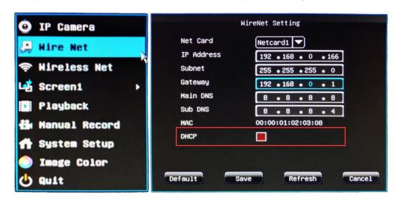
If not familiar about the LAN environment, or private network, users can turn on "DHCP", which ensures gaining IP address automatically.
